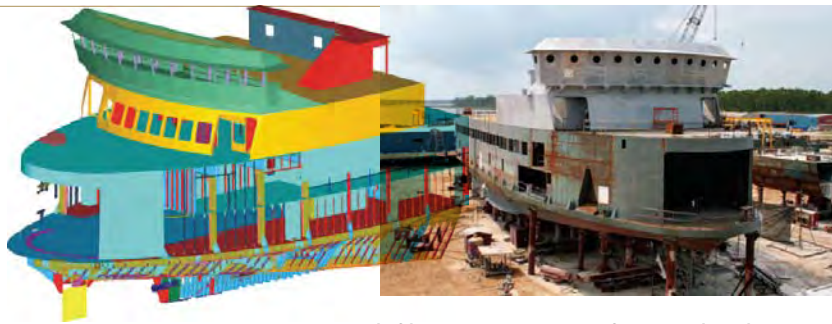
Computer-generated image (left) and actual building of the ship (right).
